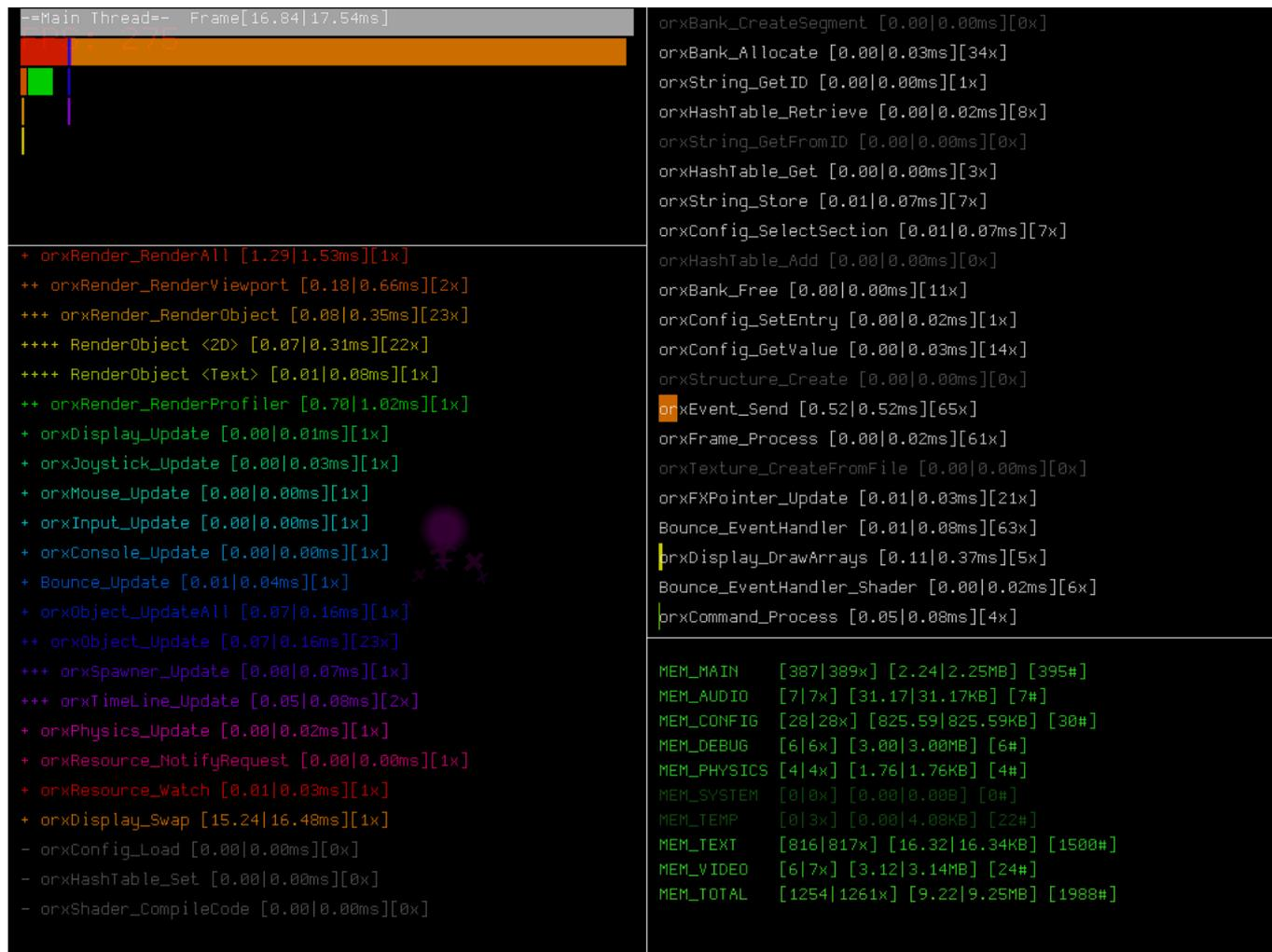
The tool helps you diagnose bottlenecks and monitor performance and internal resources.
