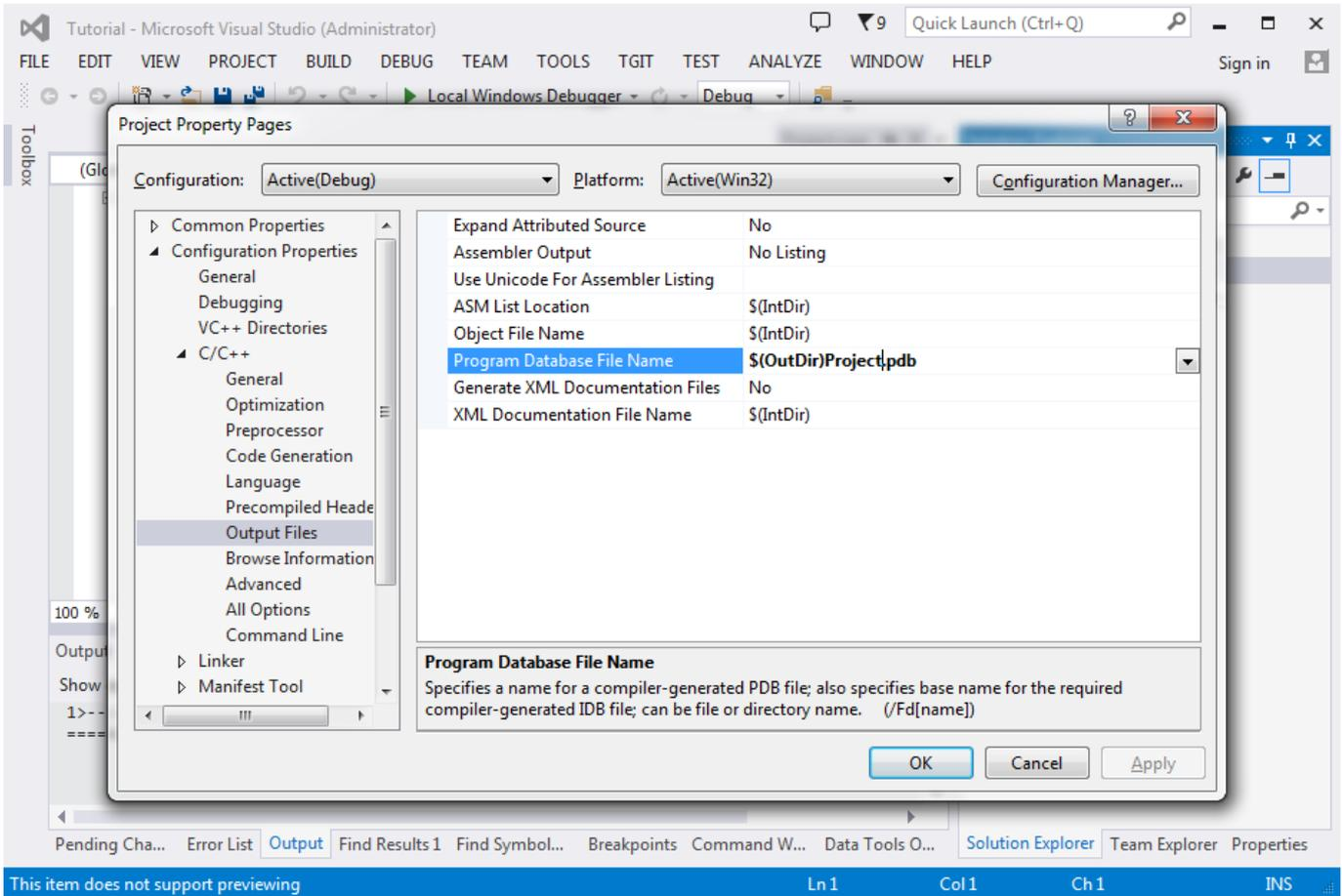
Finally, in the Linker section, change the Output File to: \$(OutDir)Project.exe so that the correctly named executable will be written to the bin/ folder:
