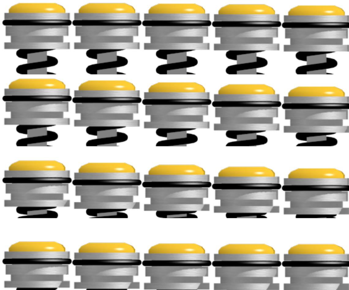
The job of this bumper is to spring up and knock away any objects that collide with it. After it has sprung up, it needs to compress down again and stay compressed until the next collision.
