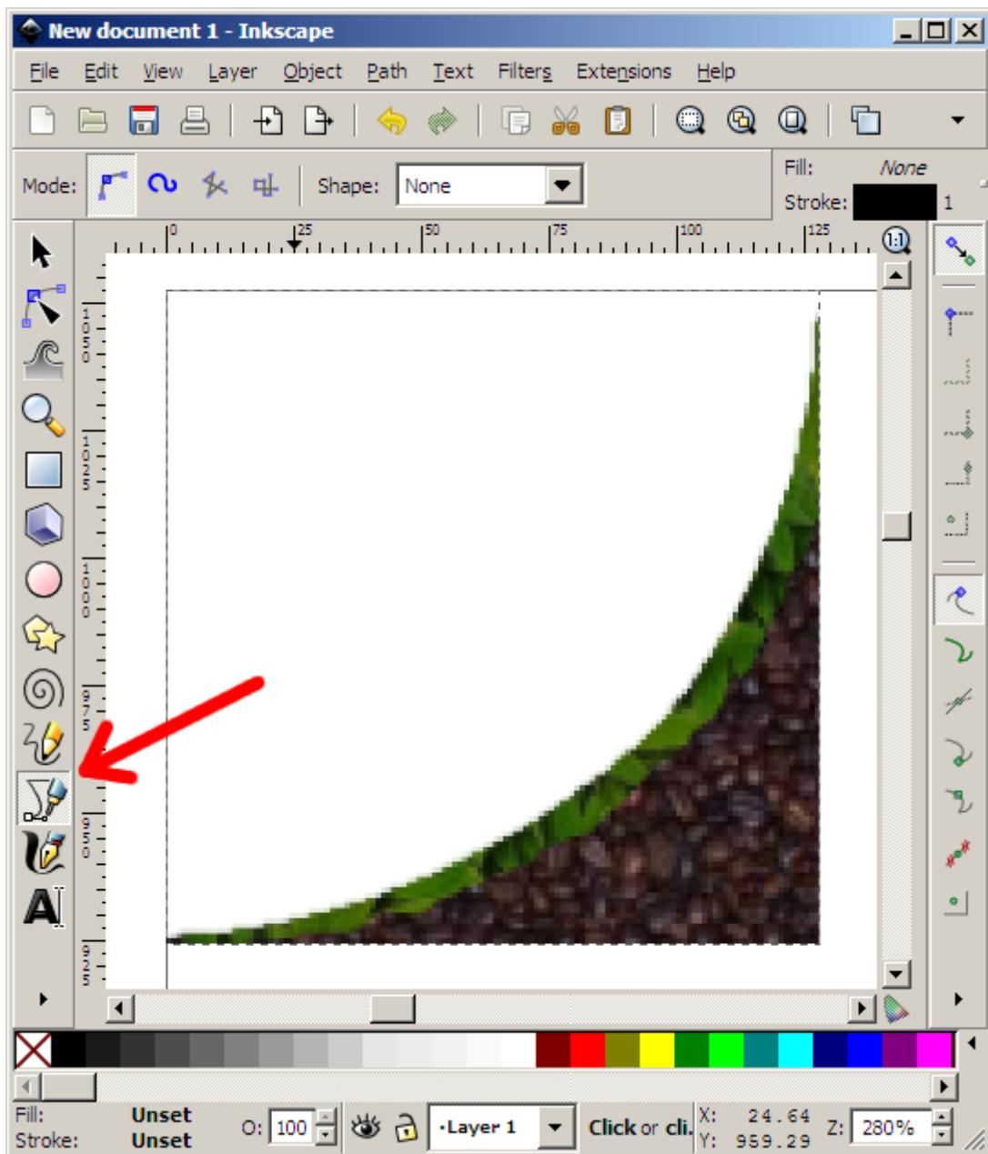
9. Draw a triangle. It must be drawn in a clockwise direction. So in this example, you could start on the left hand point, go up and right for the second point, then straight down for the third. This is drawing in clockwise which is required by Box2D in orx. I suggest you select the Fill and Stroke properties to have a nice bright stroke, and semi transparent fill to make it easy to visualise your triangles, squares or polygons.
