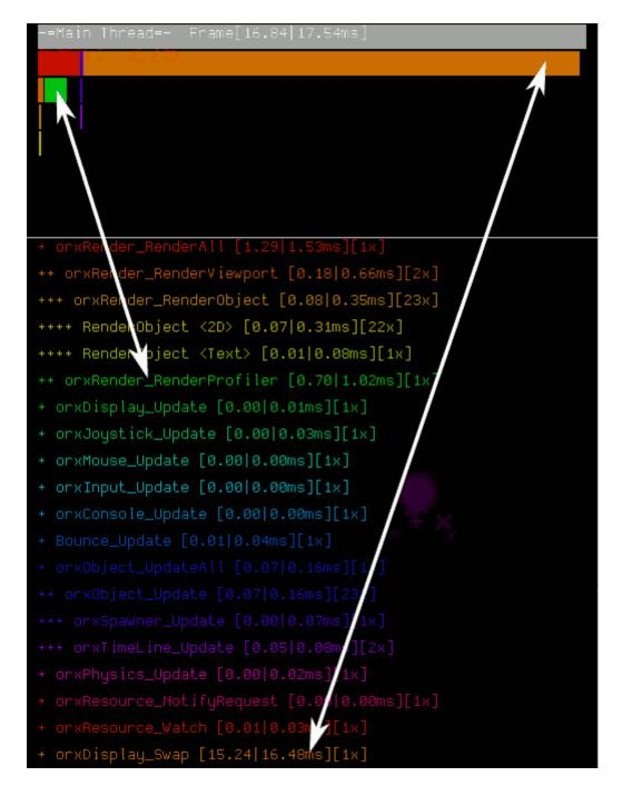
The bars are spread over four or more lines. The row of the bar corresponds to the level of the function call marker. For example, the orxRender\_RenderAll function call is on the top level, so sits in the top row. The orxRender\_RenderObject function call is three levels into the hierarchy and is therefore on the third row.
