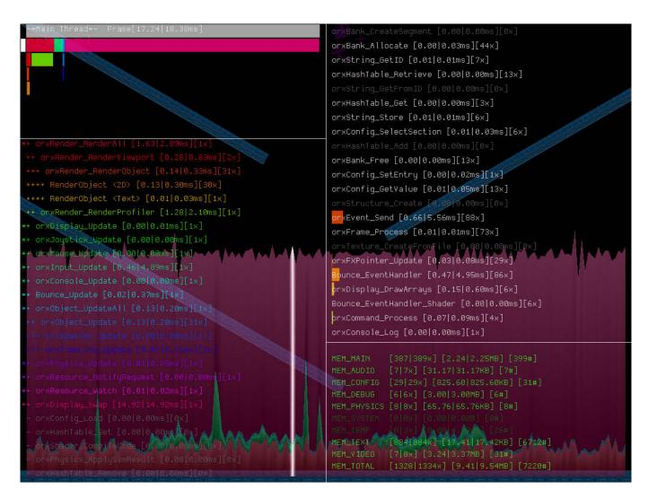
You can pause this graph with F5 and you can scroll back and forth (using the Left and Right keys) through the history to a particular frame to inspect the meters and values for each Marker to observe spikes.
